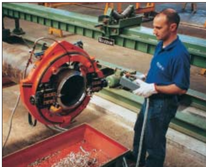
The two upper locking jaws are pre-adjustable upon standard diameters.
