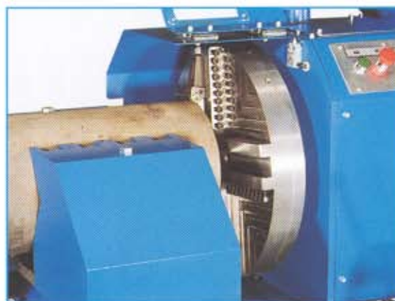
Prism clamping for pipe diameters of 60 mm up to and incl. 330 mm (FBM-12) and 80 mm up to and incl. 410 mm (FBM-16)
