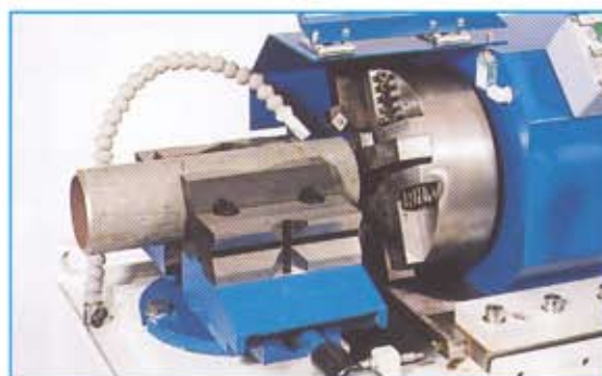
Prism clamping for pipe diameters of 46 mm up to and including 180 mm
