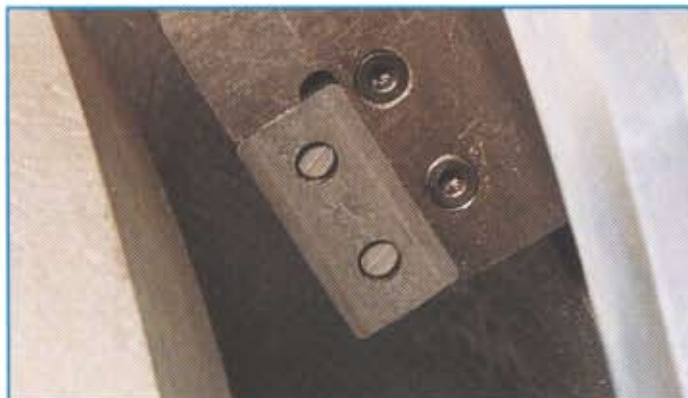
Interchangeable insertholders for inserts with a cutting length of 45 mm
