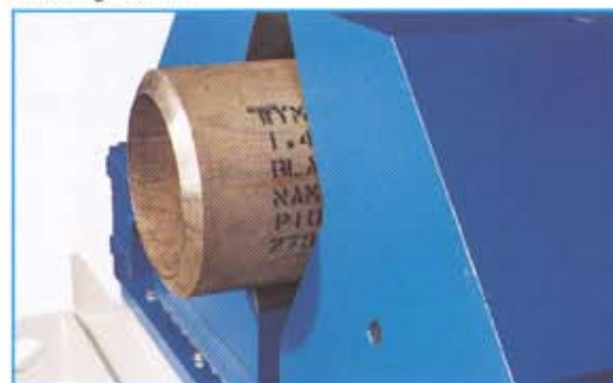
Suitable for wall thicknesses of 20 to 25 mm in one processing operation
